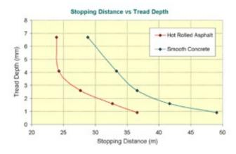
In 2003, the British Rubber Manufacturers Association (BRMA) commissioned MIRA to study the effect of tyre tread depth on braking distances. Using tyres of varying tread depths, they performed repeated stops on two different wet surfaces at 80 kph (50mph). Braking distances are evident throughout, with significant increase below 3mm.
